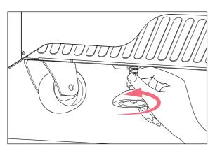
2. Rotate the leveling feet down.
