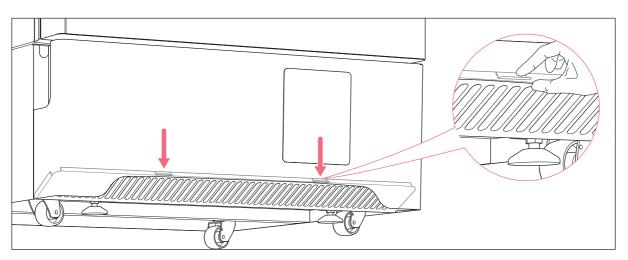
Fig. 7-1: Folding down the air intake grille
