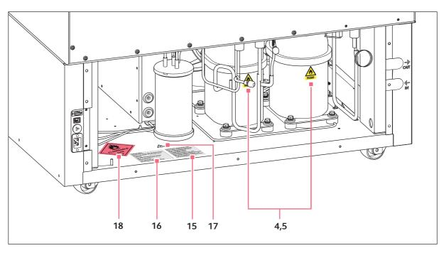
Fig. 2-2: Warning symbols on the rear of the opened device
